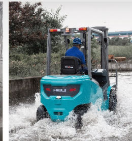
After 10mins wading test, the vehicle has no failure. (Water depth 200mm)
