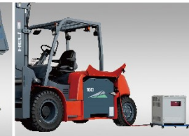
Interlocking vehicle fast charging interface
