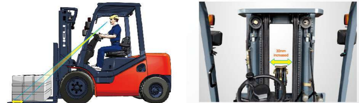
■ visibility at the fork tip and goods 20mm increased ■ front view 30mm enlarged
